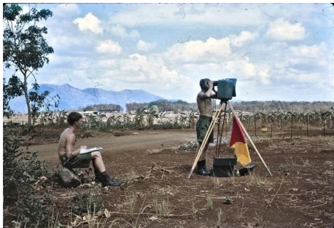
Photo at left: Clive booking, Keven Bush operating MRA2 tellurometer.
